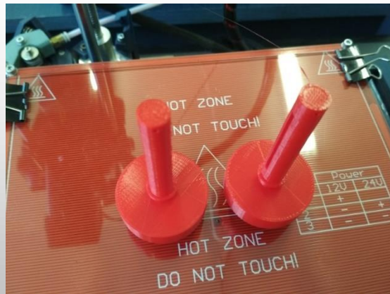
Overhangs causes poor layer adhesion, bulging and curling on the surface
