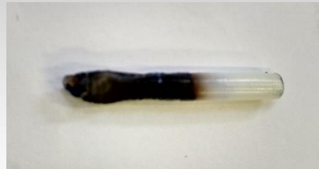
Teflon guide overheated and blocked
