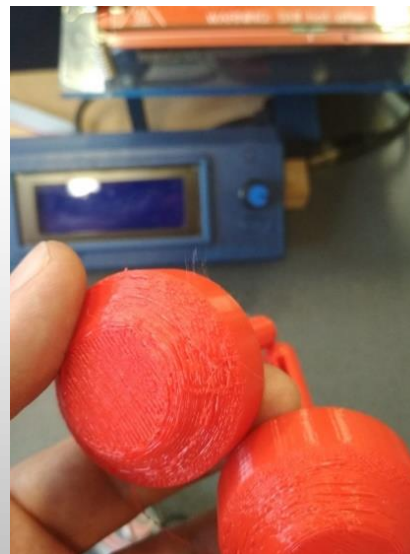
Overhangs causes poor layer adhesion, bulging and curling on the surface
